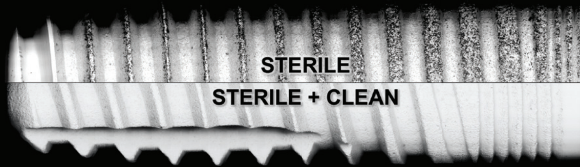
Combined SEM image of the surface of two implants, each removed shortly before from sterile packaging. Full-size resolution SEM image mapping, Backscattered electron imaging 500x.
