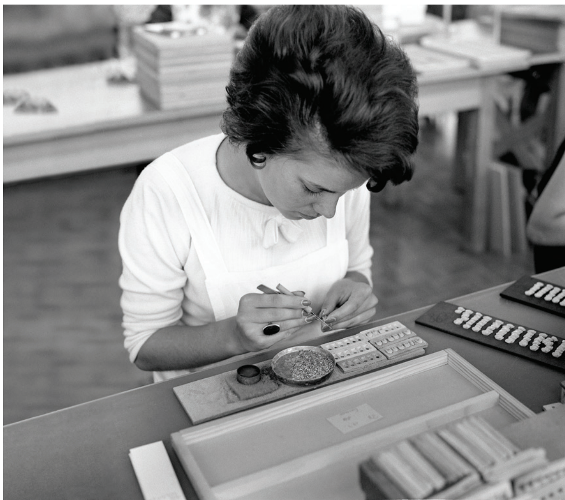
◀ An employee inserting crampton gold pins into the back of ceramic crowns. (Image: Liechtensteinisches Landesarchiv/Walter Wachter, Schaan)
