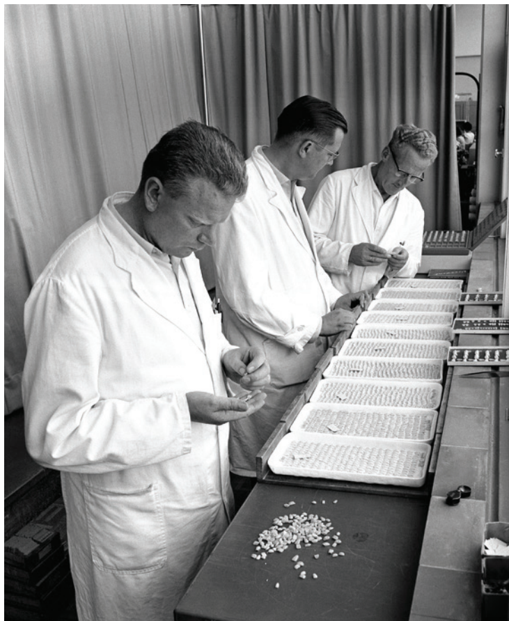
• Visual quality control of ceramic crowns after final firing. (Image: Liechtensteinisches Landesarchiv/Walter Wachter, Schaan)
