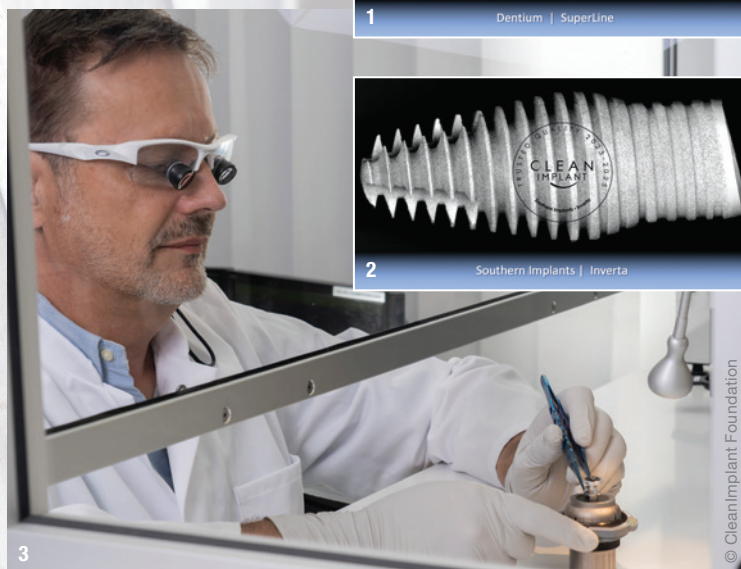
Fig. 1: SEM image SuperLine implant—Dentium. Fig. 2: SEM image INVERTA implant—Southern Implants. Fig. 3: Dr Dirk U. Duddeck placing an implant on the sample holder of the scanning electron microscope.
