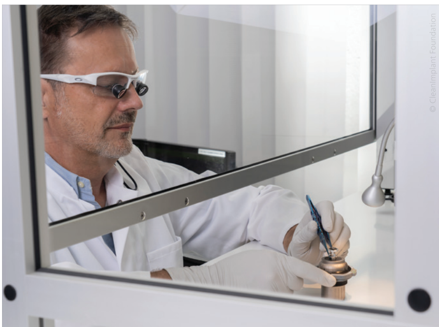
Dr Dirk U. Duddeck placing an implant on the sample holder of the scanning electron microscope.
