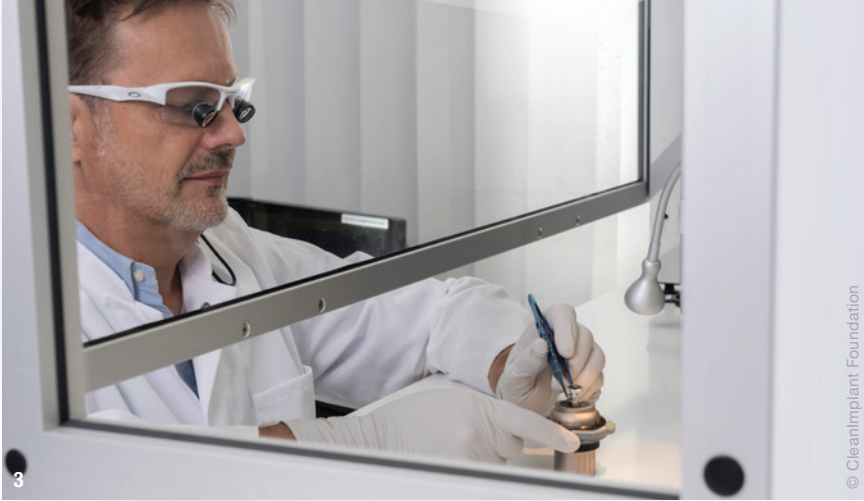
Fig. 3: Dr Dirk U. Duddeck placing an implant on the sample holder of the scanning electron microscope.
