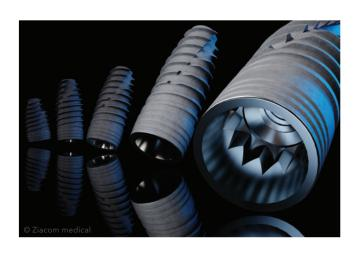
At the apical end, the implant includes an active, self-tapping, and atraumatic apex. This design element provides controlled advancement during insertion, particularly in soft bone, and helps prevent lateral or apical displacement. It contributes significantly to achieving primary stability, which is essential for both immediate and delayed loading protocols.
