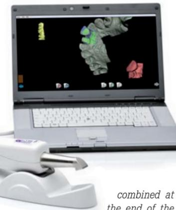
combined at the end of the process. A complete scan of the arch can also be carried out in several stages. According to MyRay, the iD3 keeps the sapphire glass of the tip at a temperature slightly higher than that of the oral cavity during intraoral scanning which is supposed to prevent condensation caused by the natural humidity levels present.
