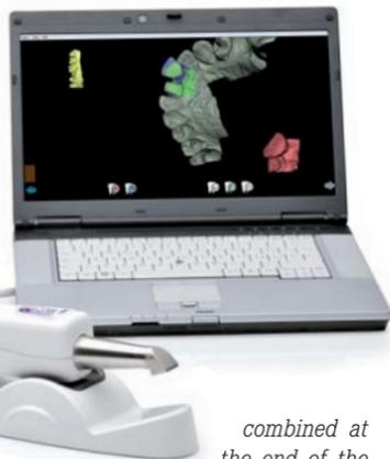
combined at the end of the process. A complete scan of the arch can also be carried out in several stages. According to MyRay, the iD3 keeps the sapphire glass of the tip at a temperature slightly higher than that of the oral cavity during intraoral scanning which is supposed to prevent condensation caused by the natural humidity levels present.
