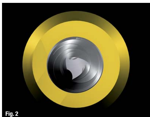
Fig. 2 _ WaveOne apical cross-section, modified convex triangular.
