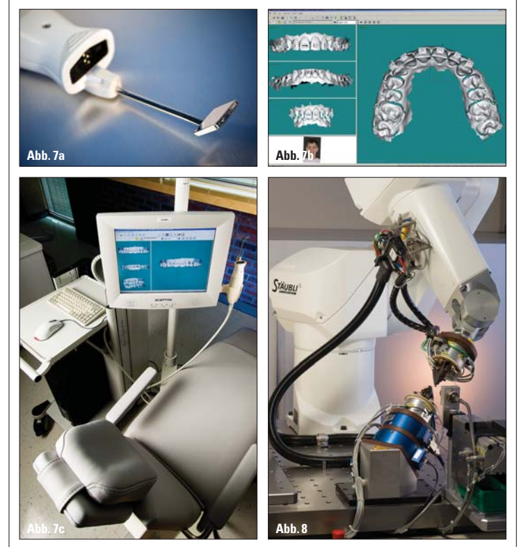
Abb. 7a-c: OraScanner-Spiegel (a), Rohdaten intraoralen Scan (b), Scanningstation am Stuhl (c). – Abb. 8: Biegeroboter.
