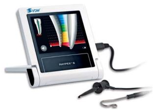
For precise length determination, RAYPEX 6 uses the latest multi-frequency technology. The 3-D graphic display constantly indicates the position of the tip of the file, while the automatic zoom-in function in the region of the apical constriction enhances safety in the critical section just before reaching the working length. Acoustic signals allow for a "blind" localisation of the apex.
