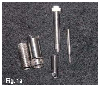
Fig. 1a_ Components of the bottle-neck device.
