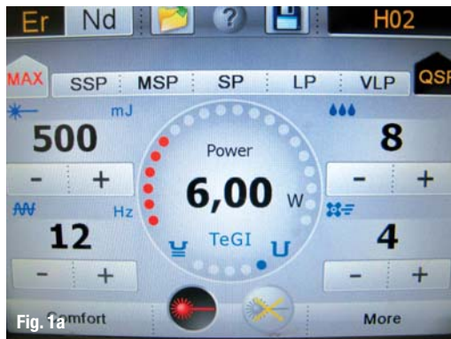
Fig. 1_a) LightWalker AT settings for QSP mode; b) H02-C handpiece; c) H14-C handpiece.
