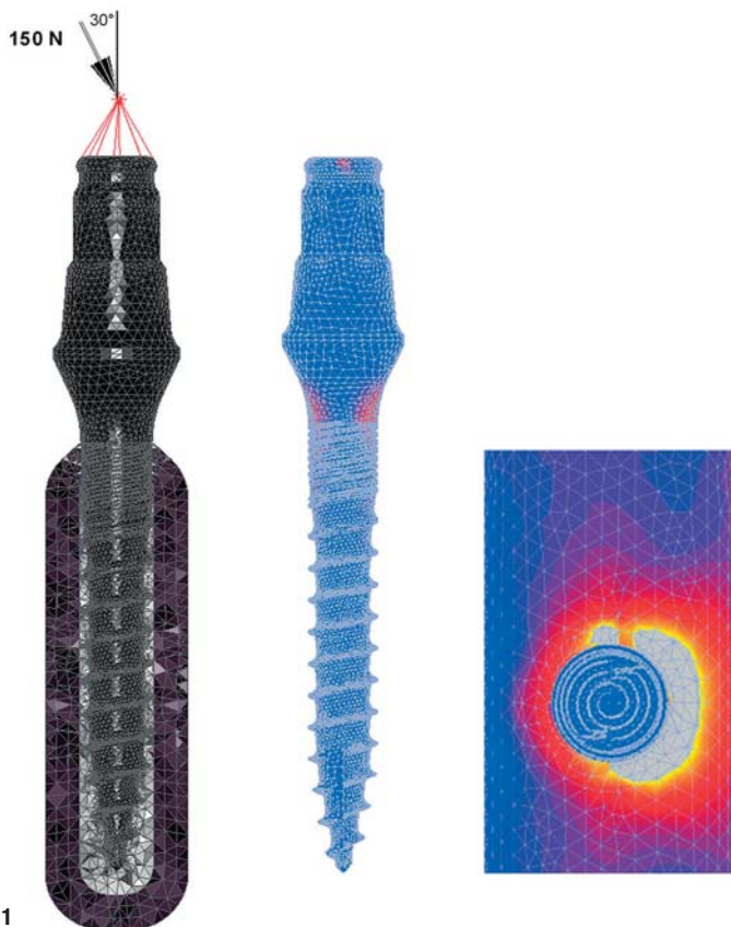
Fig. 1 _Finite element model of an experimental mini implant in an idealised bone segment of an anterior mandibular jaw (left). Calculated strains in the implant. The maximum strain level is found in the area where the corticalis is penetrated (red spots in the middle). The picture on the right shows an overhead shot of the corticalis. In the grey area, the bone is overloaded. 5
