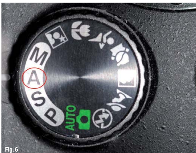
Fig. 6_Most contemporary cameras have automatic exposure setting.
