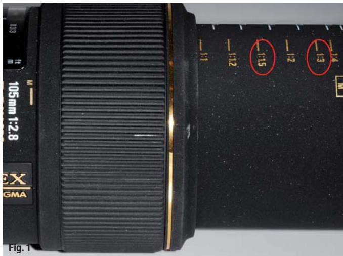
Fig. 1 _ Barrel of the lens with printed ratios.
