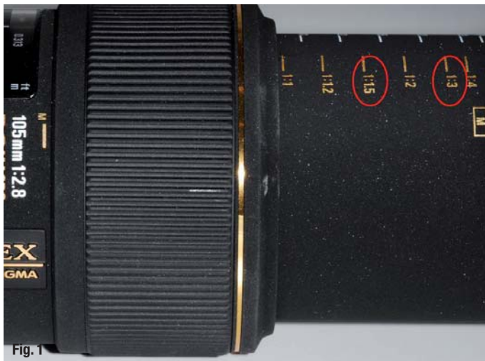
Fig. 1 _ Barrel of the lens with printed ratios.
