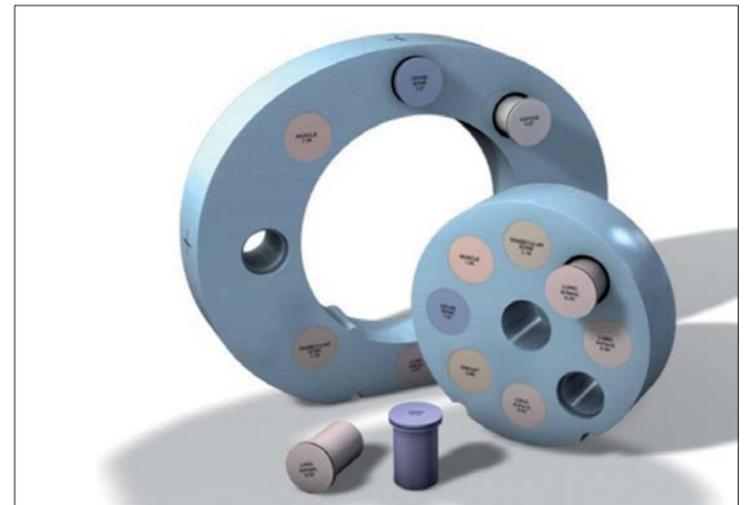
Abb. 2: Electro Density Phantom CIRS Model 062.
