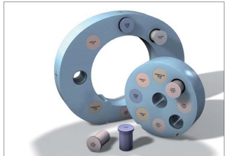
Abb. 2: Electro Density Phantom CIRS Model 062.
