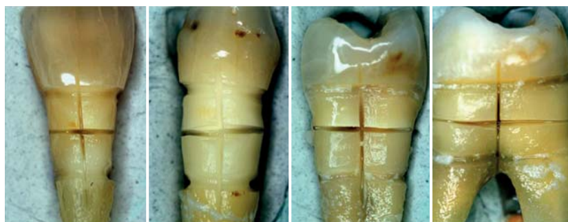
Fig. 1 Samples of (a) Incisor, (b) Canine, (c) Premolar and (d) Molar after quadrangle preparation in the tooth neck area.
