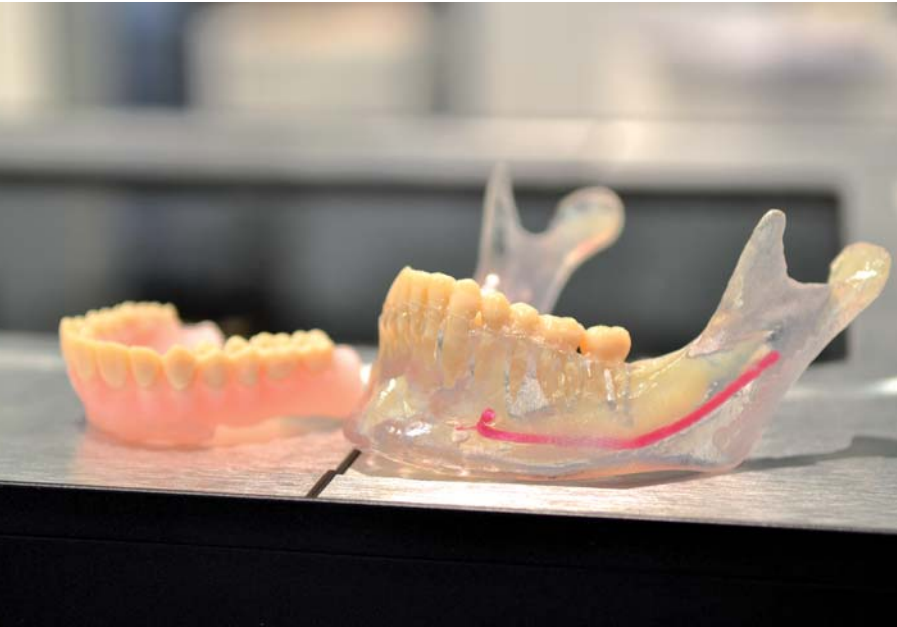
Fig. 3 Printed jaw model with high-definition tooth, root and nerve canal anatomy rendered in contrasting materials and colours.
