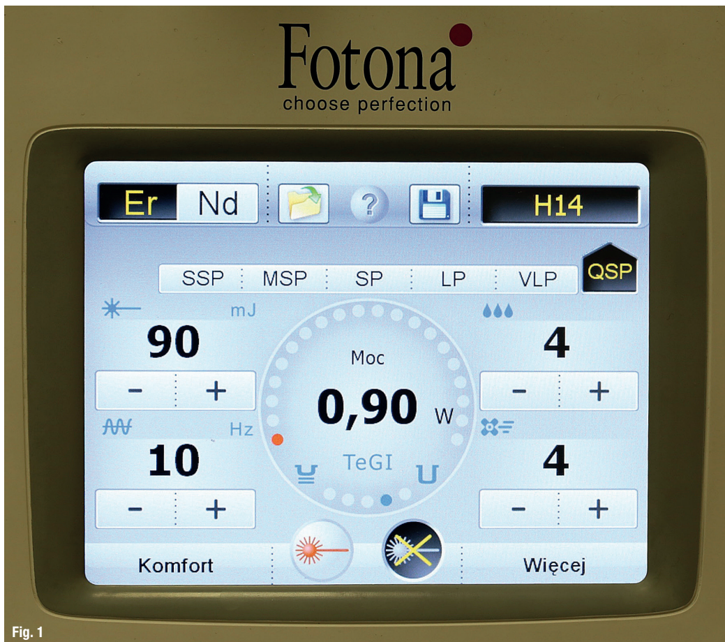
Fig. 1: Laser screen. The parameters of Er:YAG laser: H14/conical tip, QSP, 0,90 W/90 mJ, 4 W/4 A.
