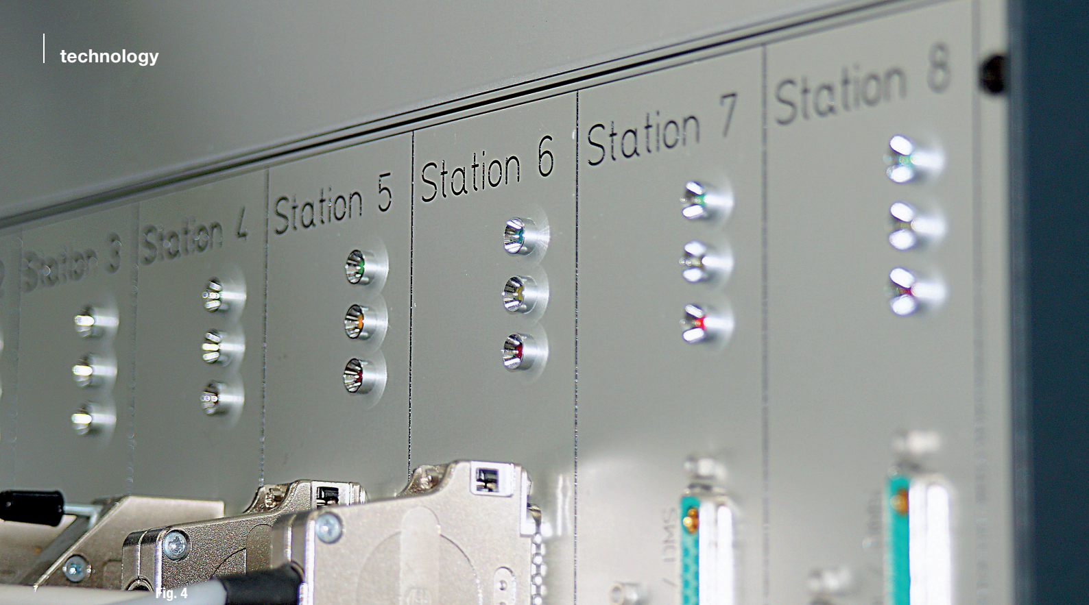
Fig. 4: Eight electronic components can be integrated into the control unit DORA CONTROL.
