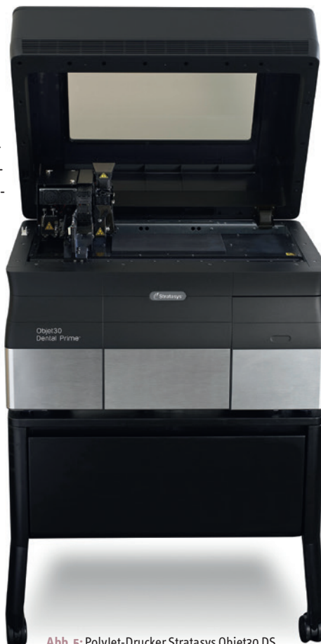
Abb. 5: PolyJet-Drucker Stratasys Objet30 DS.
