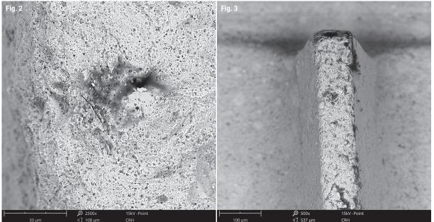
Fig. 2: Organic contamination on zirconia implant (SEM image at 2,500x). Fig. 3: Organic particles on outer thread of zirconia implant (SEM image at 500x).
