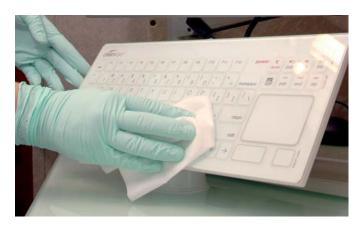
be absolutely hygienic and dust-free. Cleankeys uses touch-capacitive technology, similar to what you might be familiar with on touch-sensitive appliances such as a microwave oven or Ceran top stove. A small electric field is created above each key, which is affected by the presence of a human finger (try using the end of a pencil and you'll see it won't work). The sensors are working even when you're wearing gloves.
