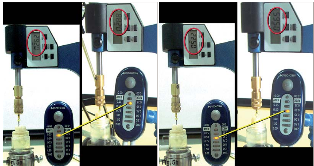
Figs. 5a & b _The MedicNRG-XFR displays extra fine resolution and very small values of distortion from the real measurements: from 12 μm (a) to 65 μm (b).
