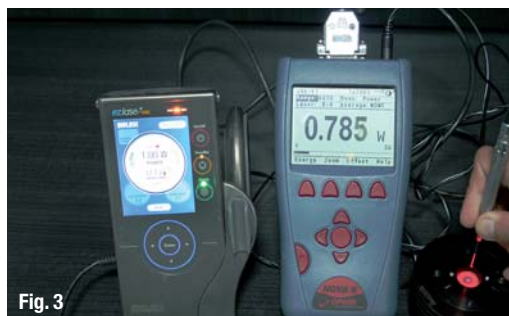
Fig. 3 The power meter measuring the power at the distal end of the tip.
