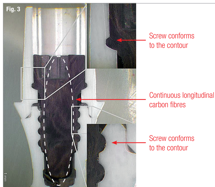
Fig. 3: The VICARBO® screw, when tightened, conforms to the contour of the internal thread of the implant.
