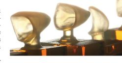
Less chipping—the outstanding machinability of Amber Mill is evident from the edges of the milled restorations
