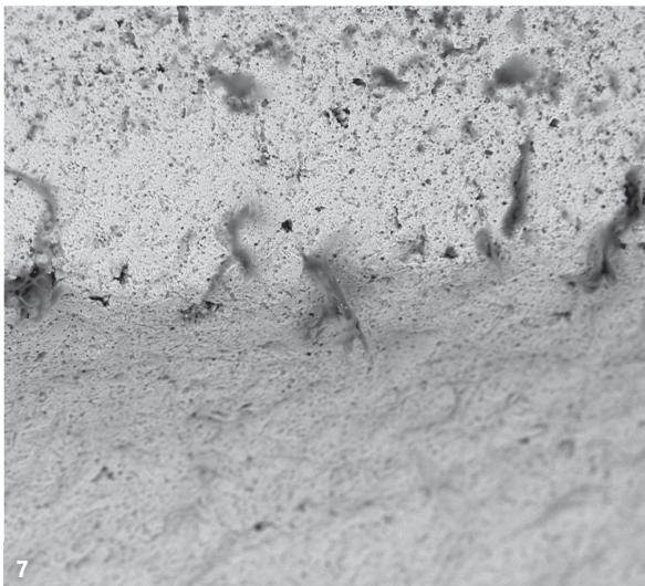
Fig. 7: Significant plastic material (polyacetal) on the shoulder of a ceramic implant (vitaclinical, VITA Zahnfabrik) from abrasion from the packaging.
