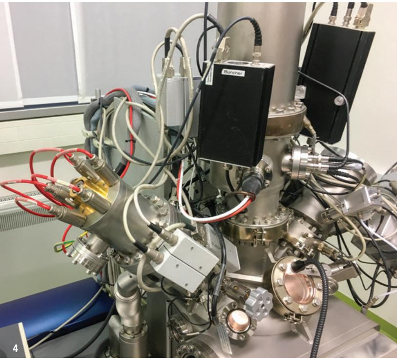
**Fig. 4:** Time-of-flight secondary ion mass spectrometry instrument (tascon).
