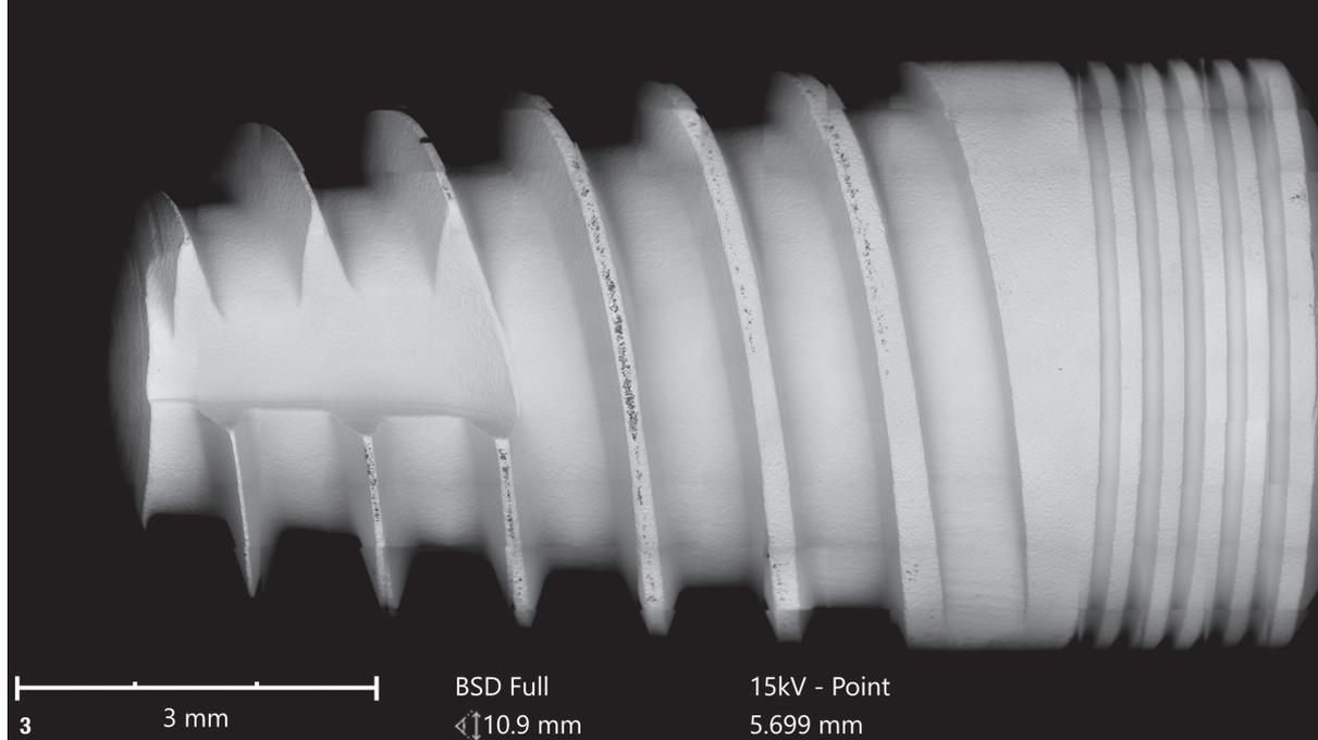
**Fig. 3:** Factory-related contamination of entire implant threads (Ritter Implants). Full-size SEM image of the implant electronically compiled from hundreds of single images at 500× magnification using the material contrast technique (back-scattered electron mode).
