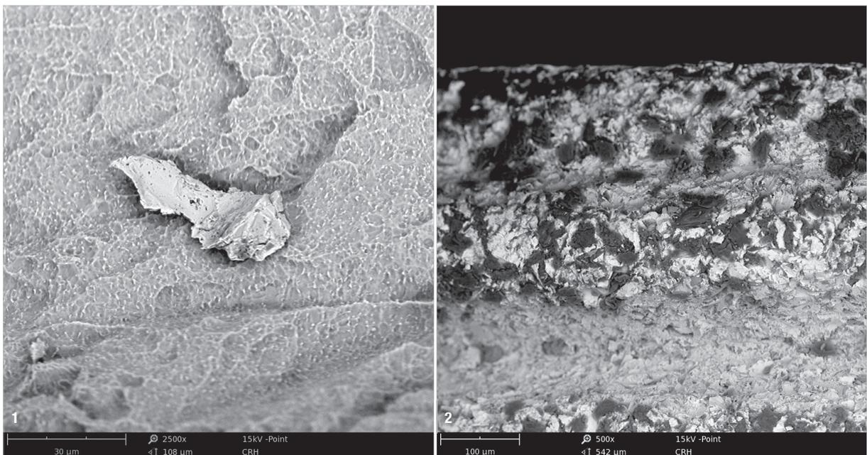
**Fig. 1:** Metal particle of iron, chromium and nickel on the surface of a titanium implant (Adin). SEM 2,500× magnification. **Fig. 2:** Numerous organic particles on the entire implant shoulder (OCO Biomedical). SEM 500× magnification.
