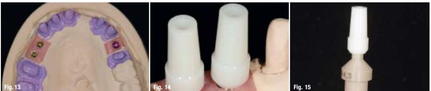
Fig. 13 Non-segmented master model with protective film. Fig. 14 Zirconium oxide sleeves in their raw form. Fig. 15 Zirconium oxide sleeves on the plastic holder, ready to be honed.
