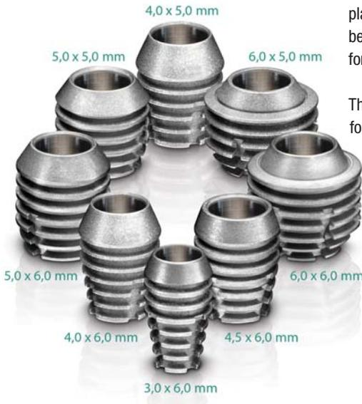
The Bicon implant design comprises plateaus, sloping shoulders and a bacterially-sealed, 1.5° locking taper implant to abutment connection. With the plateau design, cortical like bone forms around and between each plateau. This Haversian bone allows for the routine use of 5.0 mm short implants.
