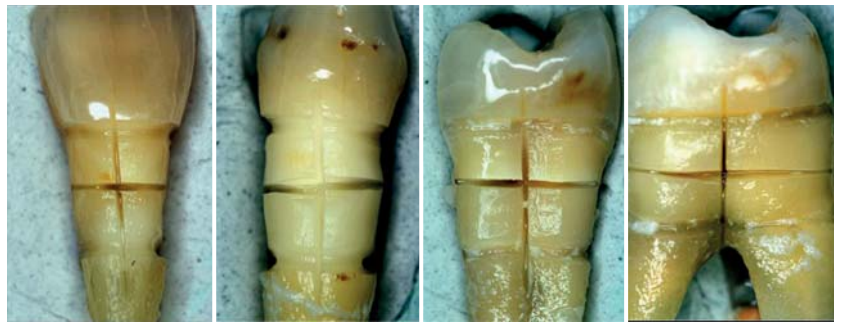
Fig. 1 Samples of (a) Incisor, (b) Canini, (c) Premolar and (d) Molar after quadrangle preparation in the tooth neck area.
