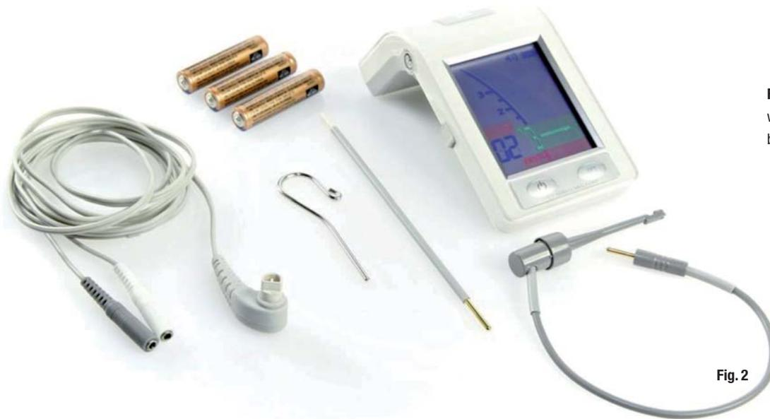
**Fig. 2** Make sure your EAL is in good working condition by checking its batteries, cords and file probes.
