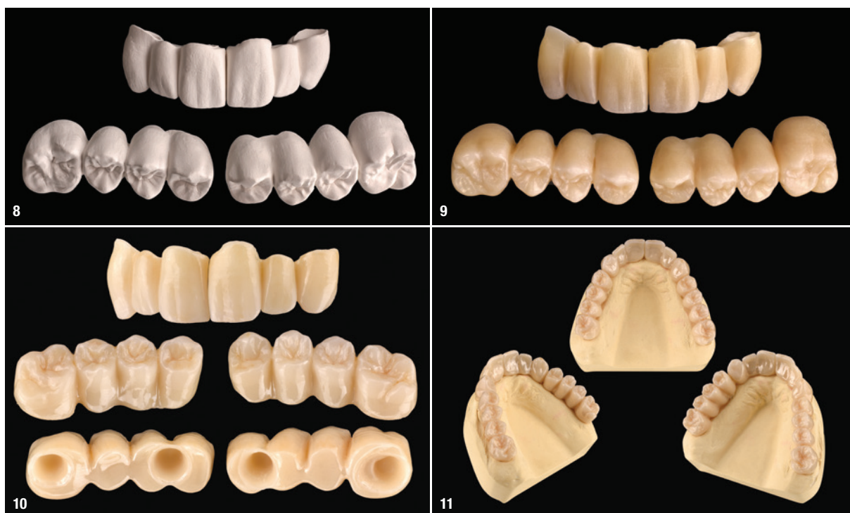
Fig. 8: Three milled bridges prior to processing. Fig. 9: Impressive aesthetics of the zirconia after the first firing. Fig. 10: Bridges after the final glaze firing and polishing. Fig. 11: Bridges on the model after the final glaze firing and polishing.
