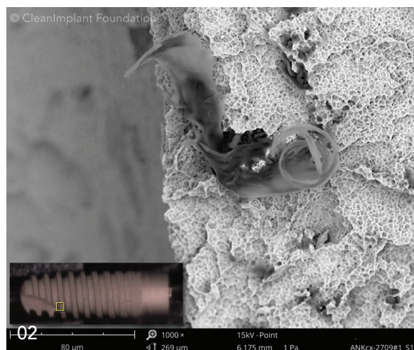
02 Same implant, different location, significant contamination: SEM image (1,000x) of plastic residues at an exposed implant thread. Additional chemical analysis identified synthetic polymers (plastic residue, polysiloxane), residues of dodecylbenzene sulfonate (a cell-toxic surfactant), aromatic and aliphatic hydrocarbons.
